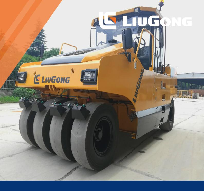
EngineShangchai SC7H180G3Rated Power132 kW (180 hp / 182 ps) @ 2,200 rpmCompaction Width2,440 mmOperating Mass26,000 kg
