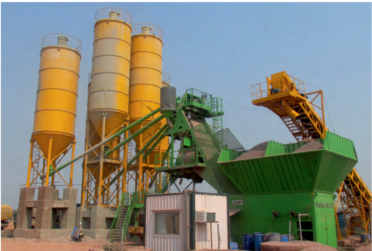
M2.25 batching plant with compartment bins with conveyor feeding option
